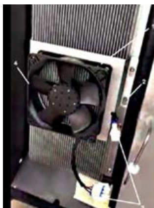
Peltier-System Cleaning (1 fan, 2 bolts, 3 cable connector, 4 fan = remove)
